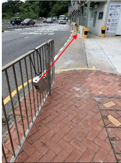
Figure 2.1 Digital dust indicator is pointed to construction site
